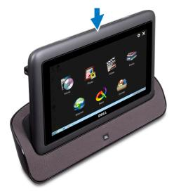
**3.** Push the tablet to connect it to the dock. Ensure that the tablet is firmly connected to the dock connector. A white power status light indicates that the tablet is docked and charging.
